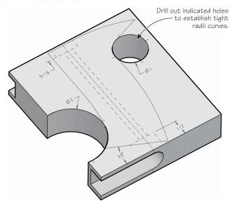
Trim the workpiece to the top and bottom contours of the handle.
