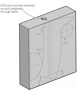
Lay out the top and bottom mortises and remove the required material.
