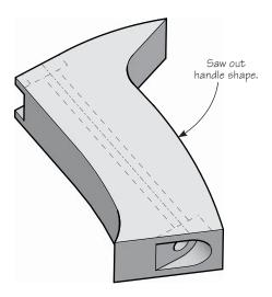
Final shaping can be done with a combination of round-over router bits, rasps, carving tools, sandpaper, etc. Proceed carefully, testing the grip often to ensure a comfortable handle. Sand the final shape smooth and finish as desired.
