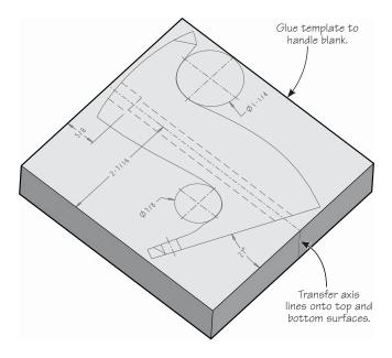
Bore out the handle rod hole. Long narrow holes can sometimes be a problem to keep aligned. It may be easier to bore halfway through from either end of the blank, providing the blank is perfectly parallel and carefully aligned in the drill press.
