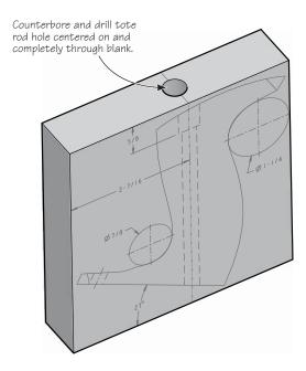
Bore out the two holes that form the tightly curved parts of the handle contour.
