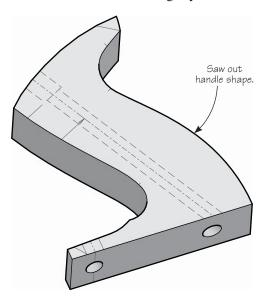
Final shaping can be done with a combination of round-over router bits, rasps, carving tools, sandpaper, etc. Proceed carefully, testing the grip often to ensure a comfortable handle. Sand the final shape smooth and finish as desired.
