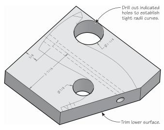
Transfer the center of the 5/16" hole onto the bottom surface and drill the hole centered on the blank.
