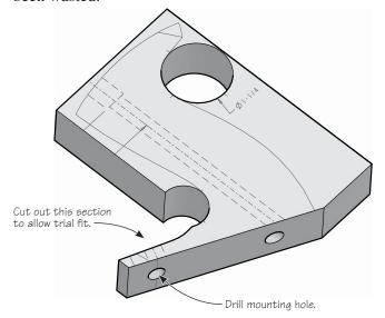
Trim the workpiece to the top, front and back contours.
