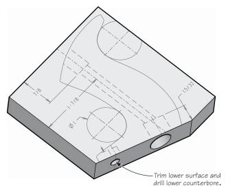
At this point, it should be possible to do a trial fit to the plane to check that the mounting details are correct. Any errors are easier to correct while the blank still has flat reference surfaces. Also, if the error is not correctable, the minimum amount of work has been wasted.
