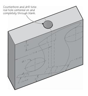
Cut the bottom surface at the indicated  $21^{\circ}$  line for a #2 tote ( $26^{\circ}$  for a #3 or #4 tote). Transfer the center of the forward hole onto the bottom surface and drill the hole centered on the blank.
