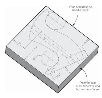
Bore out the handle rod hole. Long narrow holes can sometimes be a problem to keep aligned. It may be easier to bore halfway through from either end of the blank, providing the blank is perfectly parallel and carefully aligned in the drill press.
