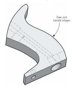
Final shaping can be done with a combination of roundover router bits, rasps, carving tools, sandpaper, etc. Proceed carefully, testing the grip often to ensure a comfortable handle. Sand the final shape smooth and finish as desired.
