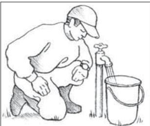
By noting the time (in minutes) it takes to fill a 5-gallon pail, gallons per hour (gph) can be calculated:
